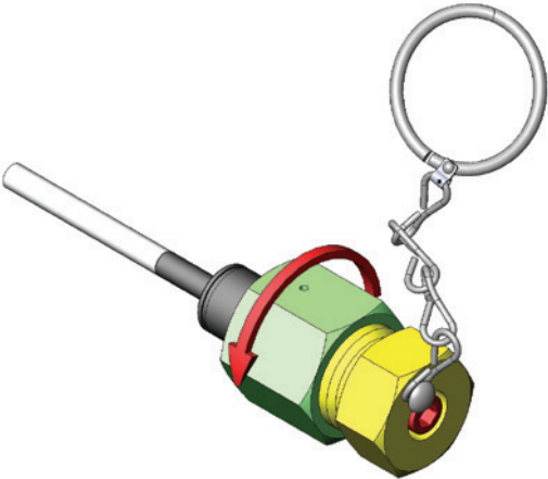
3. Assembly the nut with the plug, then tighten slightly with fingers.
